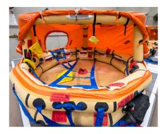
Winslow life rafts are fitted with Emergency Locator Transmitters (ELT) which automatically activate when the raft is in contact with water after opening.
